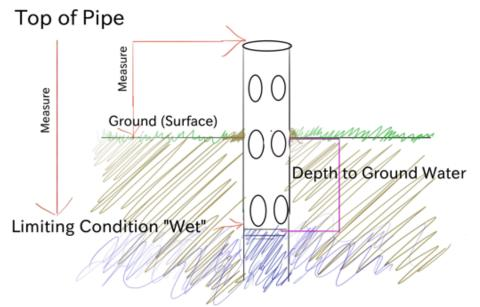
\*\*\*If there is no pipe, measure from the ground surface to limiting conditions.
